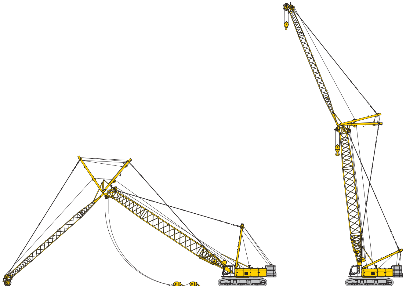
Erecting of main boom and luffing jib
